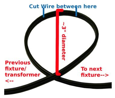
4b. In the middle of each loop, use wire cutters to cut the main line of the transformer at the top of the loop, separate the wires and strip each wire at both sides (the set of wires coming from the transformer and the set of wires leading to the next fixture).
