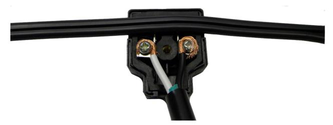
6a. Now, combine the two halves of the quick connect and tighten the screw in the middle of the quick connect. The fixture should now be connected to the main line of the transformer. If the light doesn't turn on, more often than not, there is a loose connection inside the quick connect so it is crucial that you make sure every connection inside the quick connect is secure.
