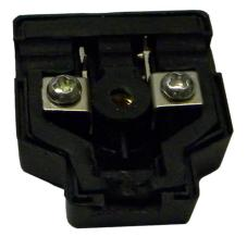
4a. Loosen the Philips head screw terminals inside the quick connect to allow for attaching the wires from the pagoda fixture. Attach one wire to each terminal (white to the left terminal, black to the right) and tighten the screw terminals to secure the wires.
